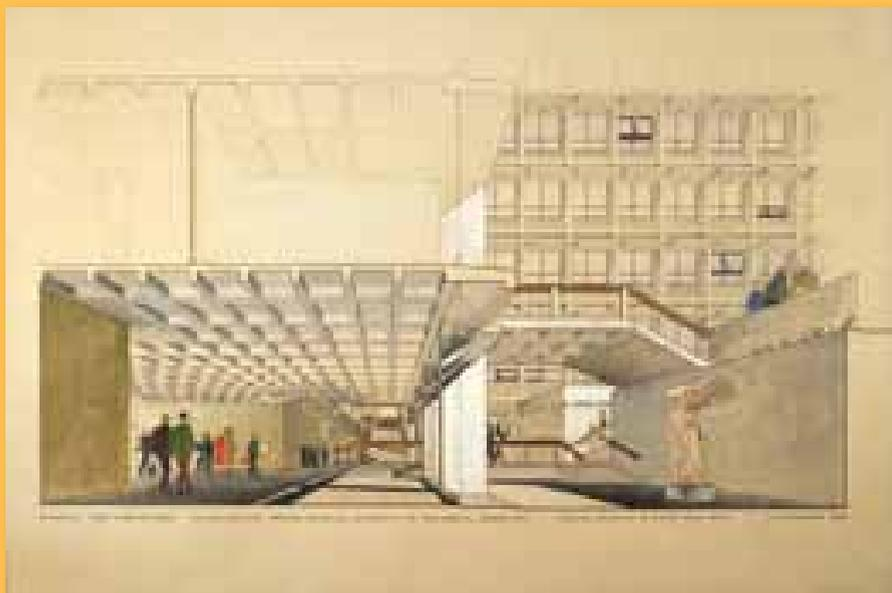
the main distribution is in the center so you have the feeling of a higher space around the periphery." Having the mechanical equipment exposed also made maintenance easier and was useful in teaching.
